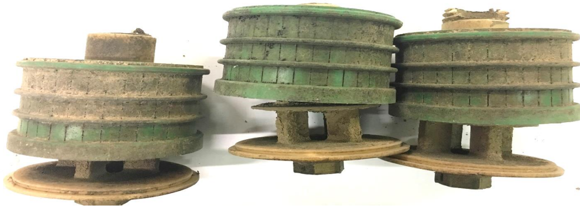
Figure 2: Examples of CaCO 3 Build Up on Nozzles
