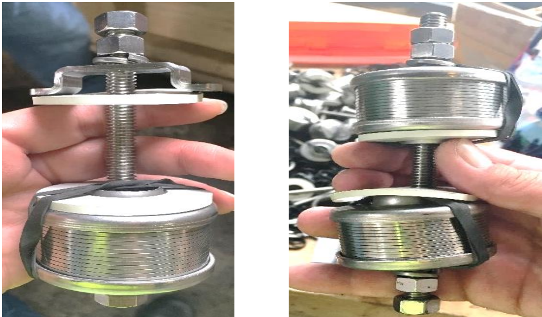
Figure 5: Stainless-Steel Nozzle Design – Top Nozzle (left), and Middle and Bottom Nozzle (right)
