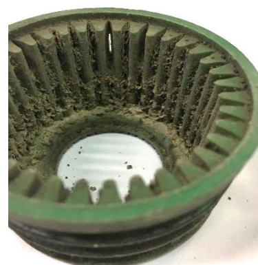
Figure 3: Interior of Nozzle with CaCO 3 Build Up
